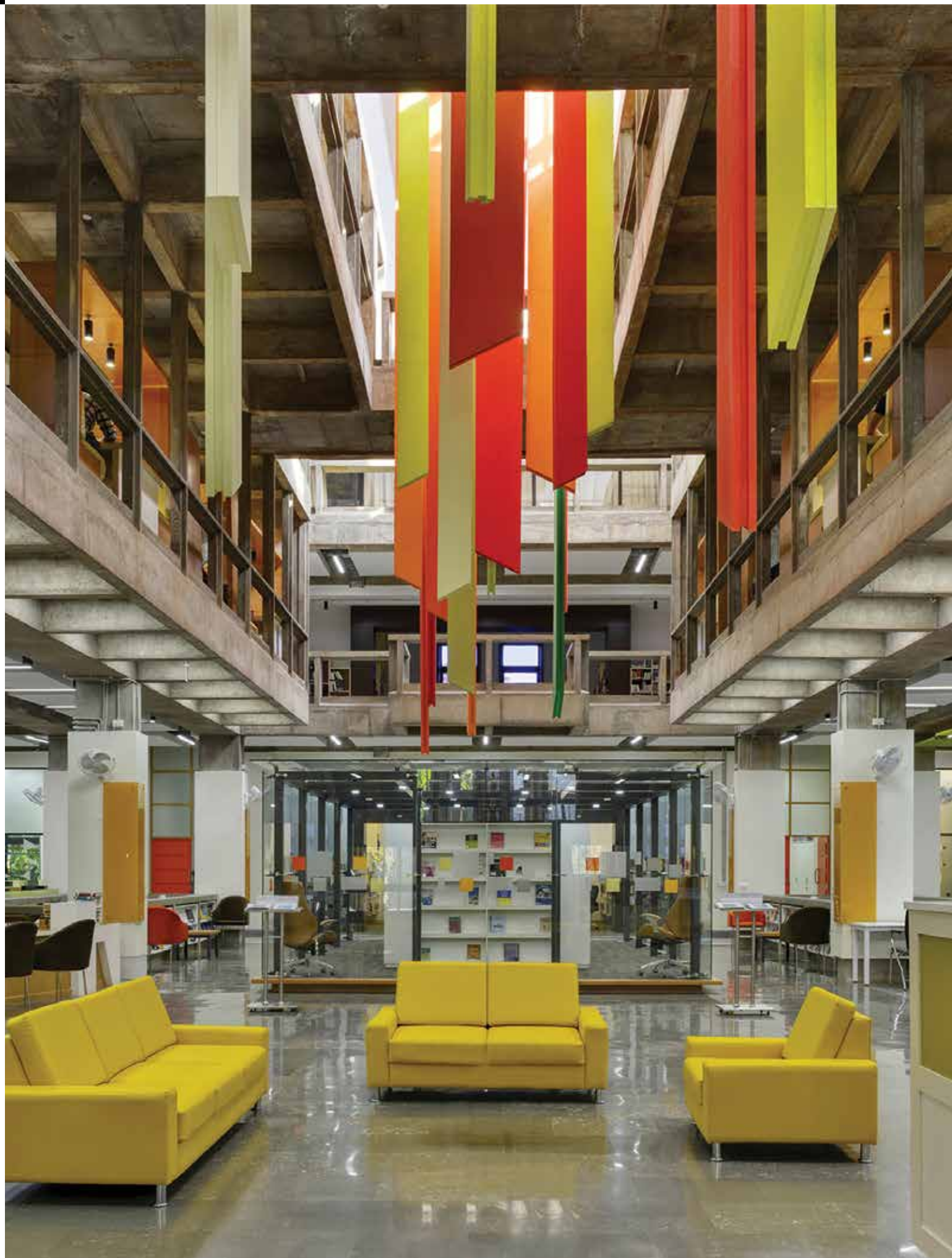
A string of colourful baffles solve the problem of acoustics.
