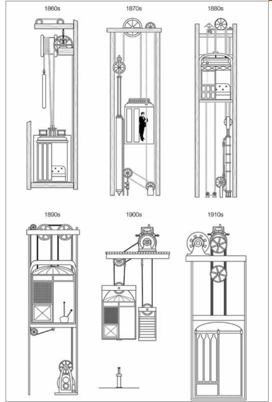
durability of the ropes to transport passengers soon led to invention of a safety break by Elisha Graves Otis in 1852 which ultimately revolutionised the vertical transport industry. Under the technique adopted by Otis, when the elevator's hoisting rope broke, a spring would operate pawls on the car which would force it to position with the racks at the sides of the shaft, resulting in the car remaining suspended in place.
