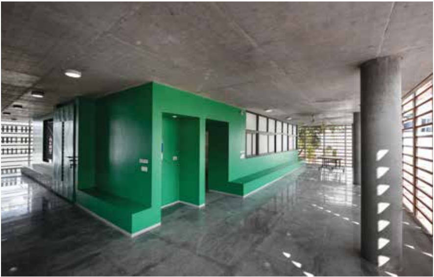
The double skin facade ensures ample natural light and ventilation sans the glare.
