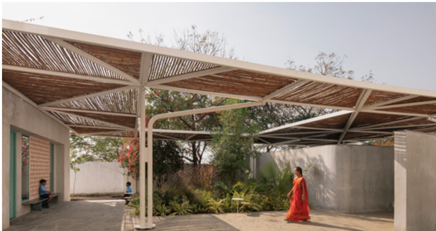
Bamboo canopy resting on metal columns serves as an excellent shading device
