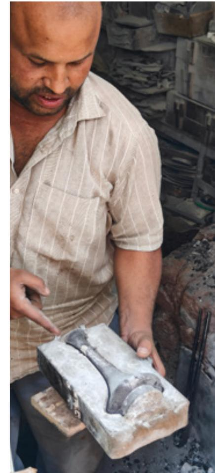
The metal piece created in the mould
