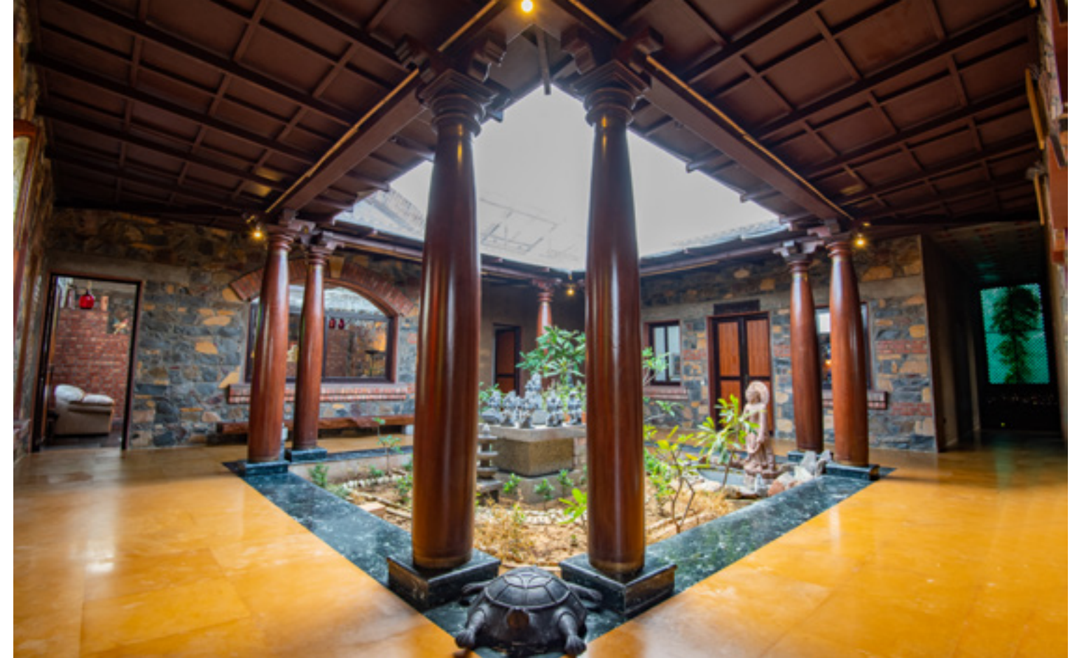
The internal courtyard, besides ushering in natural light and ventilation, creates the stack effect.
