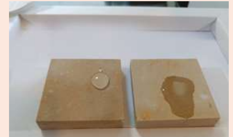
Tenax Proseal to waterproof exteriors
