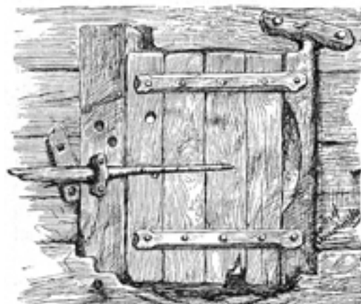
This door hinges on the stile and is called a haar-hung door. Source Wikipedia
